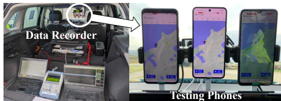
Fig. 3. NSS data collection setup during Jammertest. Left : Recording infrastructure. Right : Android phones mounted for GNSS signal acquisition during drive-test traces.
