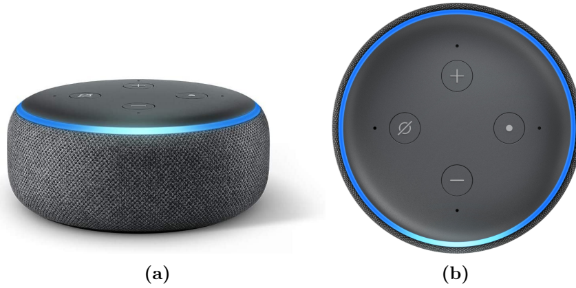
Figure 2.3.2: Amazon Echo Dot (a) and Microphones Locations (b)
